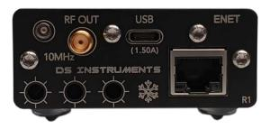
DS Instruments' various signal generator models are all designed to be as intuitive as possible, ether being controlled by the front panel, or from the USB/Ethernet interface. **Buttons and front panel modes are similar** across all models.
